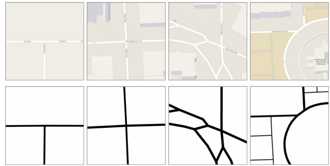
Figure 13: We use top-down stylized Google Maps (bottom row) to infer intersection complexity by counting black pixels (streets) in each scene. A higher count correlates to higher complexity.
